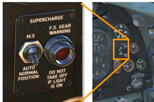
Figure 71: Supercharger control panel
