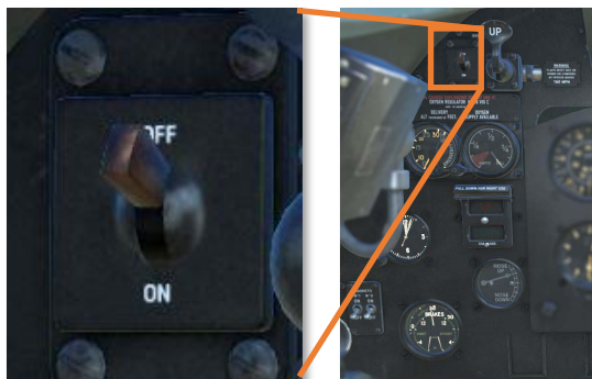
Figure 60: Navigation light control switch
