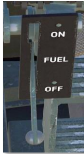
Figure 82: Main fuel valve
